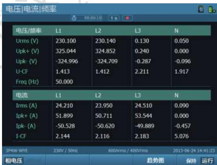
The screenshot shows the '电压|电流|频率' (Voltage|Current|Frequency) table mode interface. It displays two tables of data for three phases (L1, L2, L3) and a neutral line (N). The top table shows voltage and frequency data, and the bottom table shows current data. The status bar at the bottom indicates '3P4W-WYE', '230V / 50Hz', '600Arms / 400Vrms', and the date '2013-06-24 14:41:23'. Buttons for '相电压' (Phase Voltage), '趋势图' (Trend Chart), '保持' (Hold), and '运行' (Run) are visible at the bottom.
