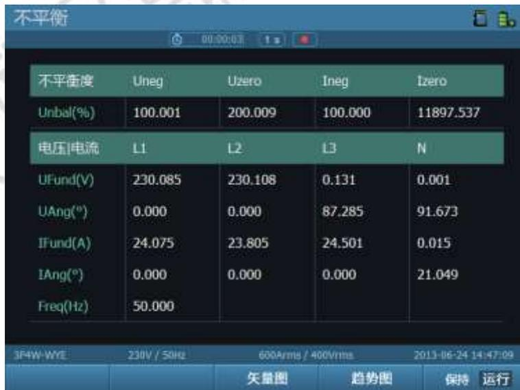
The screenshot shows the '不平衡' (Unbalance) table view. It displays a table with unbalance degrees and fundamental values for phases L1, L2, L3, and N. The status bar at the bottom shows '3F4W-WYE', '230V / 50Hz', '600Arms / 400Vrms', and '2013-06-24 14:47:09'. Buttons for '矢量图' (Vector Diagram), '趋势图' (Trend Diagram), '保持' (Keep), and '运行' (Run) are visible at the bottom.
